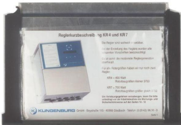
The KR4 and KR7 control units and their central component, the frequency inverter, permit you to fully adjust the rotor speed for the entire permissible range.
